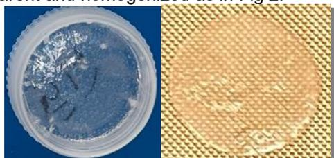
Fig2. Appearance of monolith ionogel (left) and thin ionogel on separator (right)
